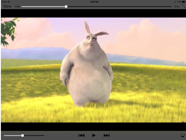
Fig. 2. Default controls of a mobile video player as used on the Apple iPad. In the lower part of the screen we can see fast-forward/reverse and play as well as volume control (which, however, can be controlled by other means, e.g., hard buttons, as well). In the upper part of the screen we can see the seeker-bar to be used for navigation by scrubbing. All controls are usually hidden during playback and need to be enabled by a tap gesture.
